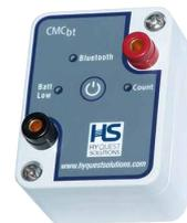
**Pulse Counter CMCbt:** Bluetooth pulse counter providing an interface between the TBRG's Reed Switch output and the FCD-App calibration software used in conjunction with HyQuest Solutions' Field Calibration Device FCD.
