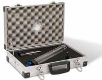
**Portable Field Calibration Device (FCD):** enables field technicians to run functional tests and calibrations of any given rain gauge in the field avoiding dismantling of Tipping Bucket Rain Gauges, reducing downtime and thereby saving time and money.
